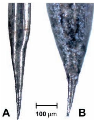
Figure 1. Optical microscope image of a platinum microelectrode before (A) and after (B) the coating process.
